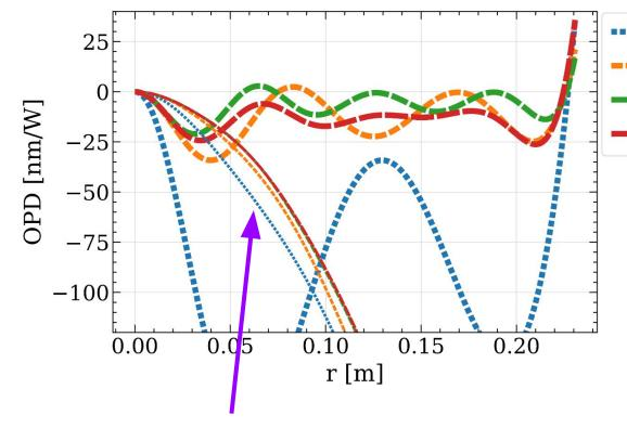
Residual surface deformation could be problematic → static mirror surface polish
