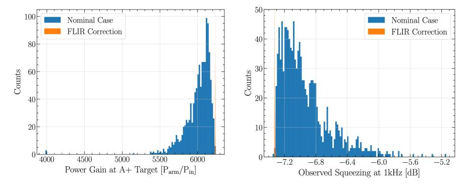
Monte-Carlo simulation (1200 trials) and results in Power Gain (Left) and the observed squeezing (Right) for the <u>nominal case</u> (5mm and 1%) and the <u>FLIR correction case</u> (0.5 mm and 0.1 %)
