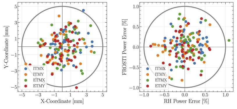
Monte-Carlo simulation with <u>randomly miscentered beam</u> <u>positions</u> on the test masses (Left, with  $3\sigma = 5$  mm), and RH/FROSTI <u>power uncertainties</u> (Right, with  $3\sigma = 1\%$ )
