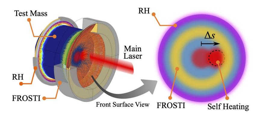
From FLIR thermal imaging of the <u>front surface temperature</u> to decode the <u>thermal state of the test mass</u>, including the RH, FROSTI power and main laser power/location
